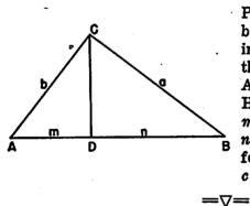
Over 90 proofs of the Pythagorean theorem have been published. The following is Legendre's proof. In the figure, triangles ABC, ACD, and BCD are similar. Hence, n/a = a/c and m/b = b/c, so that  $a^2 =$ nc and  $b^2 = mc$ . Therefore,  $a^2 + b^2 = nc + mc =$  $c(n + m) = c^2$ .
